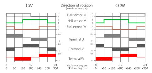
The colors of the 3 Hall sensor signals correspond with the 3 colors of the Hall lead wires.
