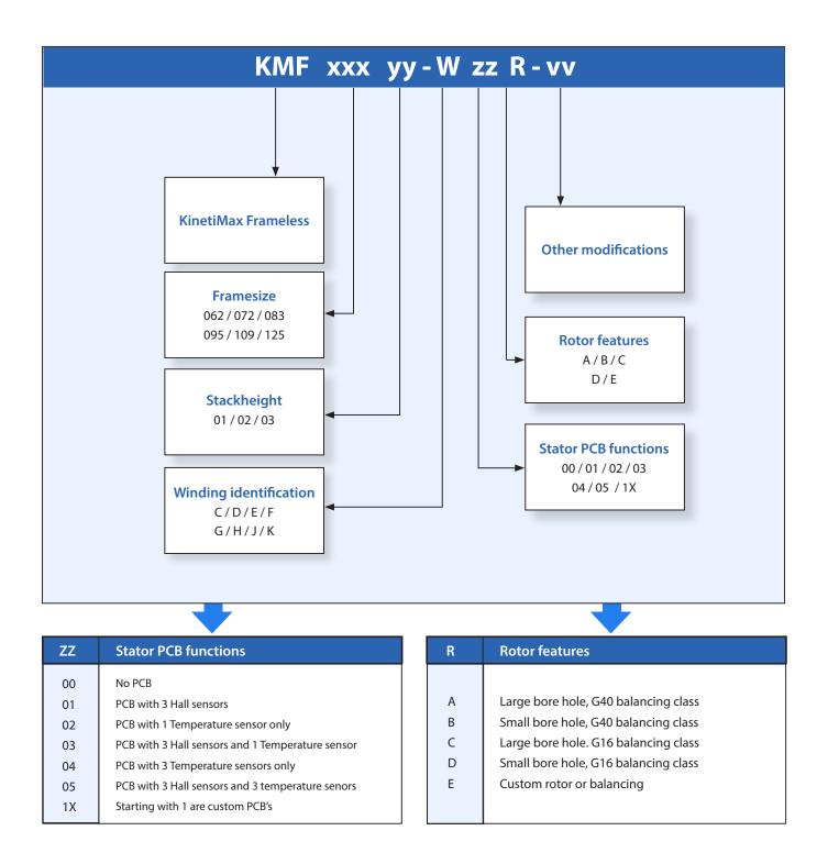
With **Other modifications** are meant custom added parts to stator or rotor like a stator bracket, other leadwires with connector or a rotor nave/shaft etc.
