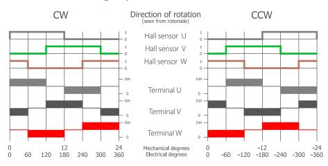
The colors of the 3 Hall sensor signals correspond with the 3 colors of the Hall lead wires. The colors of the 3 signals of the terminals U, V, W, correspond with the 3 colors of the motor lead wires.
