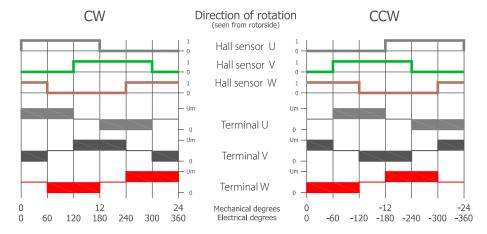
The colors of the 3 Hall sensor signals correspond with the 3 colors of the Hall lead wires. The colors of the 3 signals of the terminals U, V, W, correspond with the 3 colors of the motor lead wires.
