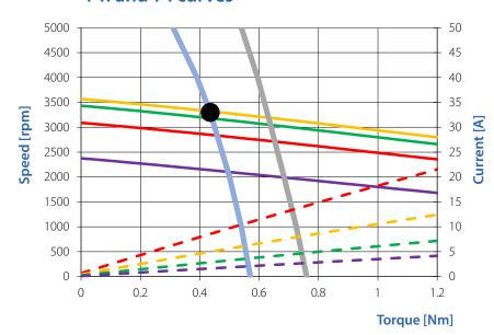
Supply current is the DC current taken from the DC power supply by the drive. The torque-speed curves and torque-current curves are made assuming a FOC drive is used.
