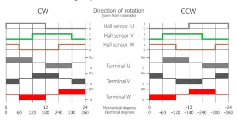
The colors of the 3 Hall sensor signals correspond with the 3 colors of the Hall lead wires. The colors of the 3 signals of the terminals U, V, W, correspond with the 3 colors of the motor lead wires.
